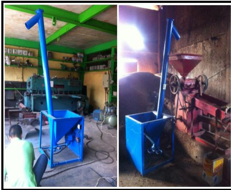
Figure 2.2. Actual Design of Screw Conveyor as Ergonomic Intervention for Material Handling
