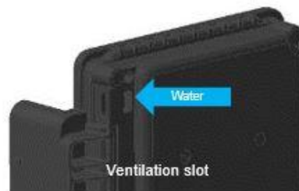
Figure 5. Ventilation slot where water through in vehicle
