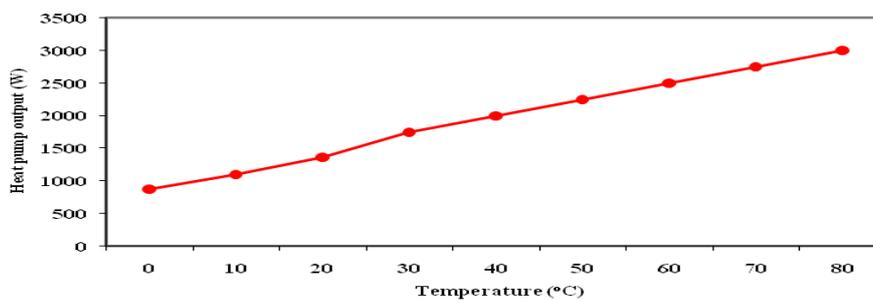
Figure 20. Variation of heat pump output with temperature.
