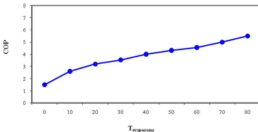
Figure 6. Heat pump performance vs evaporation temperature.
