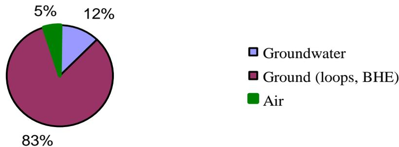
Figure 21. Distribution of heat sources for heat pumps (for space heating).
